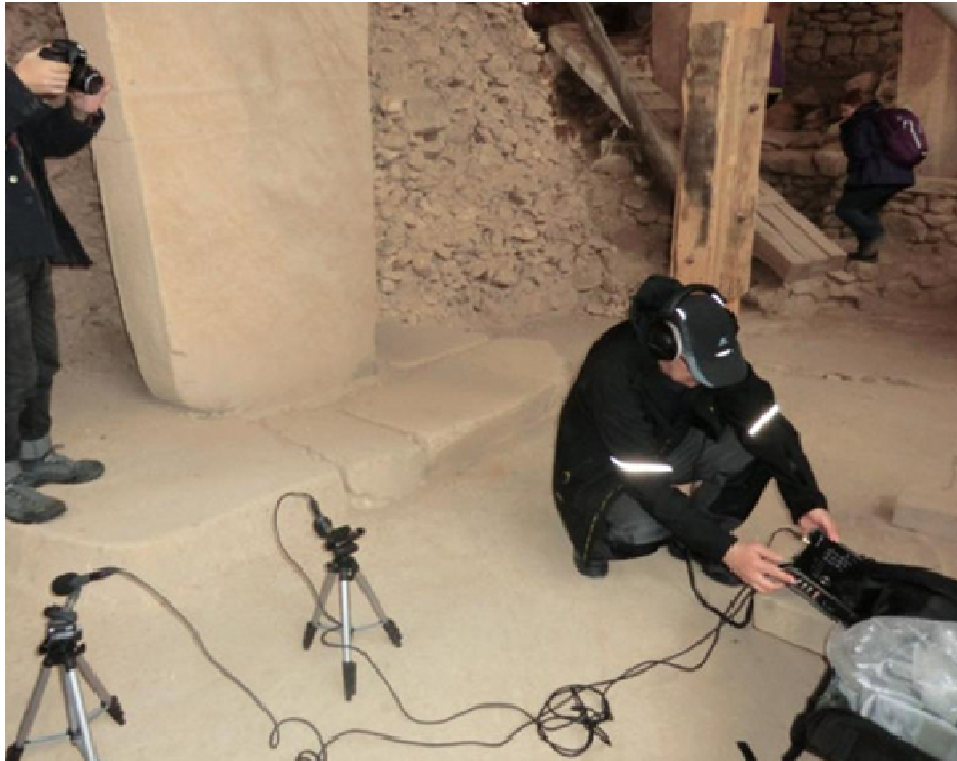
Fig. 21: We placed the microphones close to the limestone floor near the base of pillar n.18.
