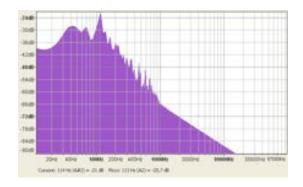
**Figure 8** – The typical aspect of resonance at 114Hz found in Hal Saflieni Hypogeum in Malta. The resonance was stimulated by a sciamanic drum, but if the drum were drummed by soft hand instead of by a ram there were no resonance by the environment (Debertolis et al. 2015).
